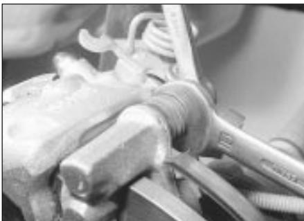
4.29 Unscrewing the forward caliper guide pin bolt
