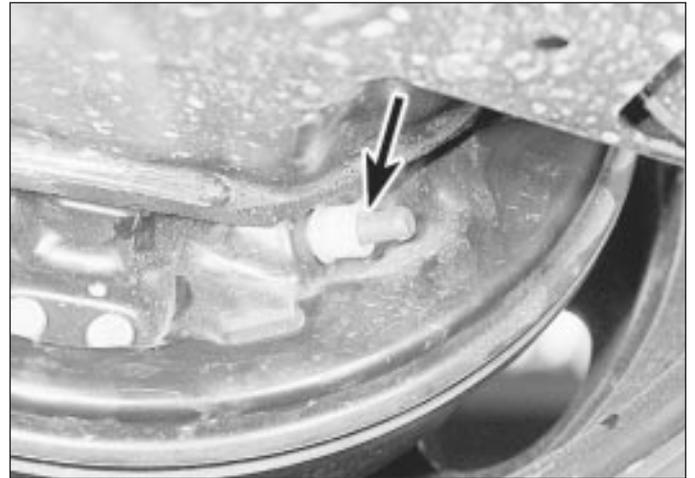
28.5 Plastic plunger (arrowed) in brake backplate
