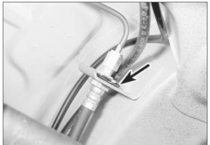
26.1 Flexible hose-to-rigid pipe union. U-shaped retaining clip arrowed
