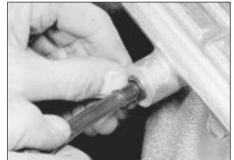
14.10 Disconnecting a later-type brake servo vacuum hose
