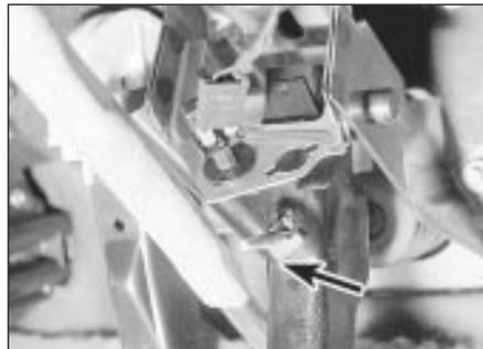
14.4 Remove the clip (arrowed) from the servo pushrod
