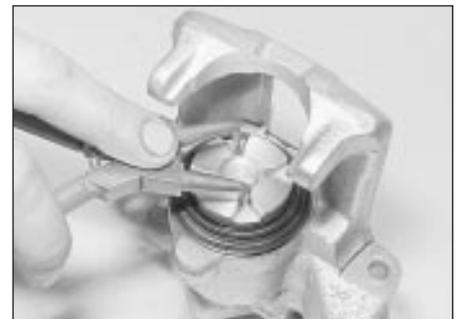
4.32 Retracting the piston using circlip pliers
