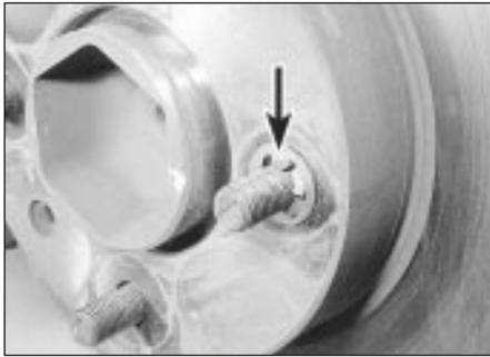
5.5a Brake drum retaining spire washer (arrowed)
