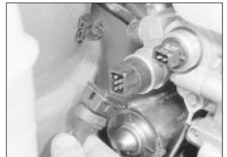
16.3c . . . and the pressure switch multi-plug - ABS
