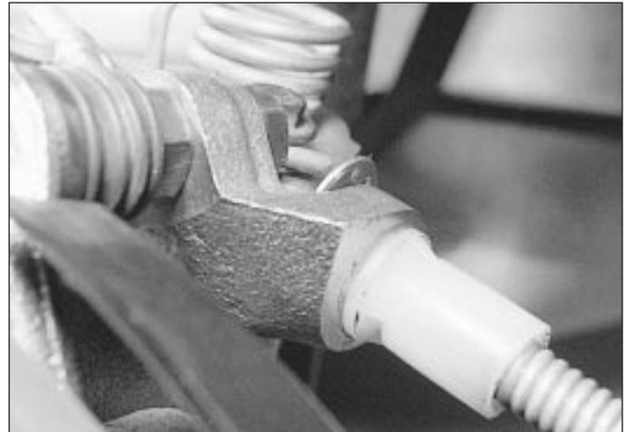
27.5b Handbrake cable-to-caliper carrier bracket attachment - ABS
