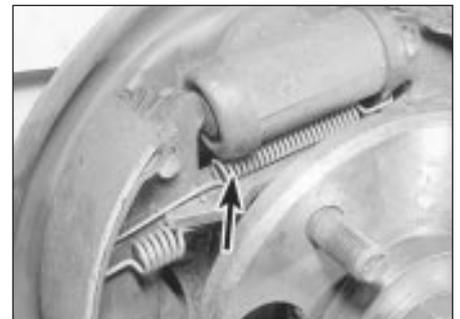
5.6a Top shoe return spring (arrowed)
